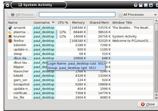
Clicking on the icon to the left of the entry box will bring up the System Activity window, where you can view all the active tasks currently running on your system. From here, you can highlight a running task, and click on the "Kill Process" button at the top left of the screen. This is helpful if you have a runaway process that's trying to bring your system to it's knees.
